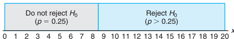
Figure 10.1: Decision criterion for testing p = 0.25 versus p > 0.25 .
